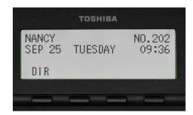
IP5000 4-line LCD display in Idle Mode
